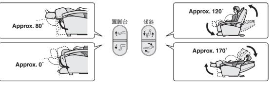
\*The reclining operation is a function that adjusts the angle of the backrest and legrest. Avoid using it for any other purposes,
