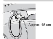
Fix the controller cord with the fastener for securing the controller cord at a position about 45 cm from the connected part of the controller on either the right or left side
